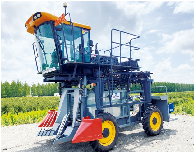
The first self-propelled blueberry (honeyberry) harvester in China
